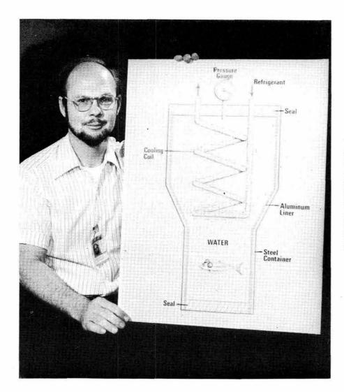
TOM PREVENDER (1255) displays a drawing which illustrates his recentlypatented method for bonding a thin aluminum liner to a steel case. The case is filled with water, sealed, and a cooling coil forms ice inside. Resulting hydrostatic pressure effectively makes the bond.
